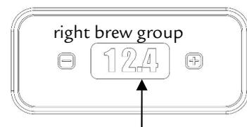
Temperature display steam boiler (t<sub>2</sub>, here 124°C) dot in the 2<sup>nd</sup> position
